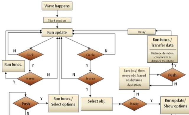
Figure 2. The algorithm controlling UI using arm gestures recognition.
